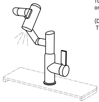
Turn on angle stops, turn the faucet on and check for leaks.
